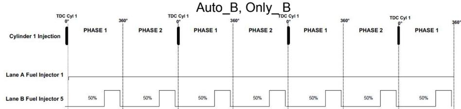
A single revolution of the engine is defined as one PHASE of the injection process.
